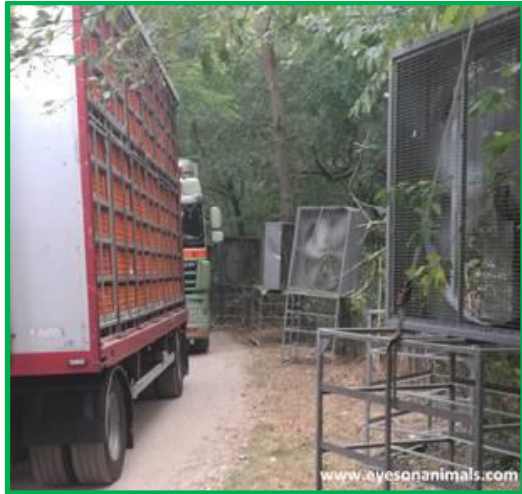
Large mobile fans to ventilate stationary trucks help reduce heat-stress
