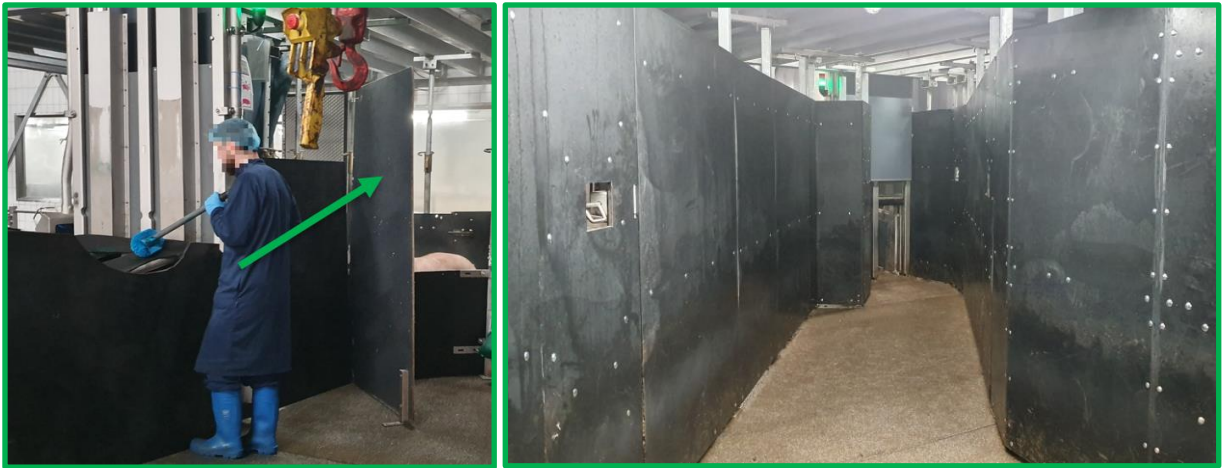
Left photo: Worker positioned behind a high, solid wall so that pigs entering the single-file raceway (from the right in the photo) cannot see him. Right photo: solid and high walls are placed all along the crowdpen to ensure that pigs cannot see moving objects or other distractions that may scare them while being moved through. Photos taken at Compaxo slaughterhouse in Zevenaar (NL).
