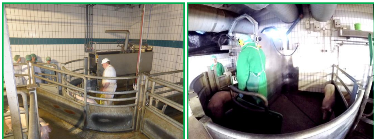
Corral shaped double entrance raceway for pigs at Naturverbund (left) and Grossfurtner (right)
