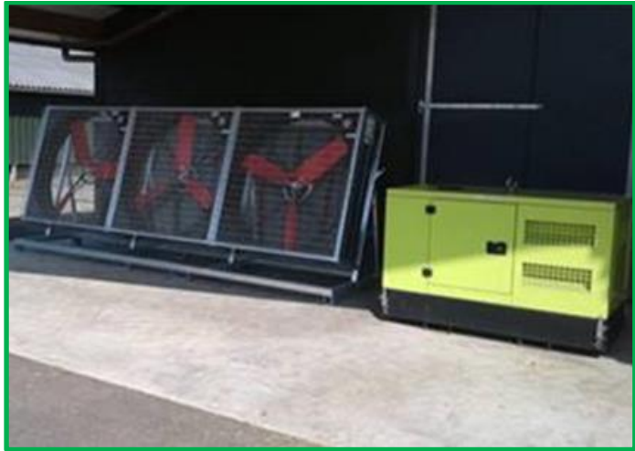
Large mobile fans to ventilate stationary trucks help reduce heat-stress
