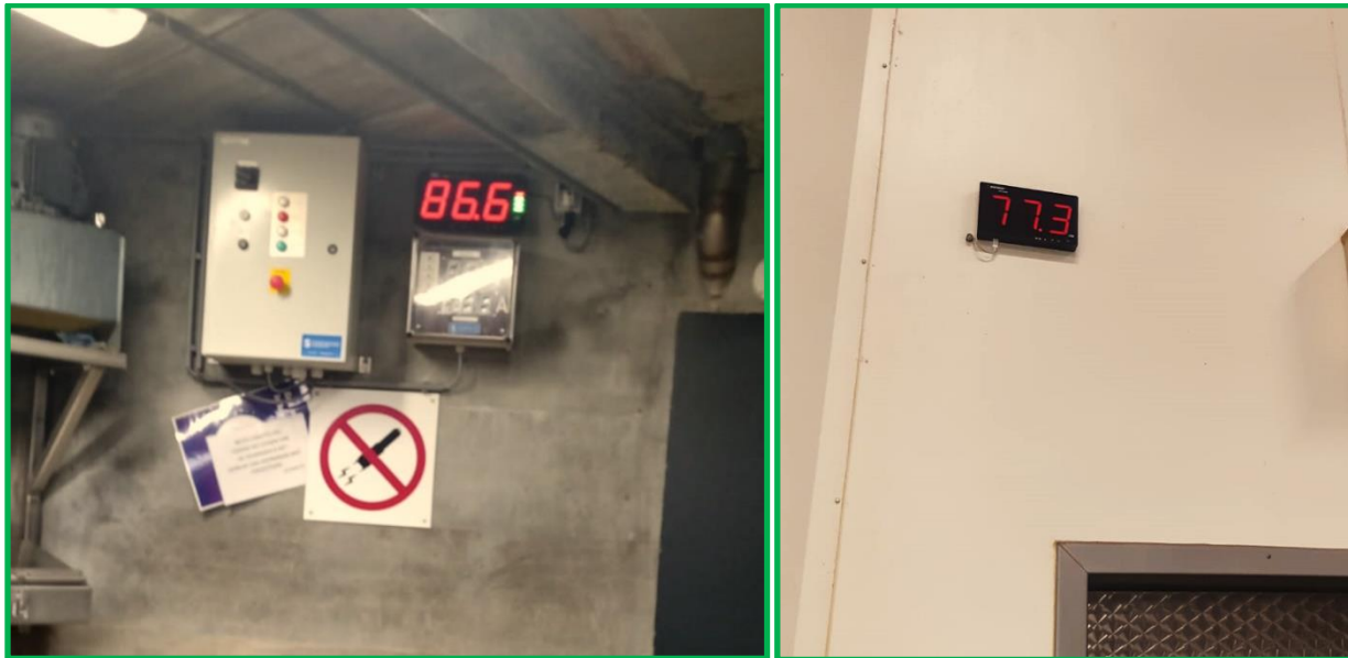
Monitors showing the decibel level in a Dutch slaughterhouse. Left: dB monitor at the unloading dock, right: dB in the lairage.
