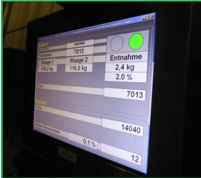
At Tönnies there is a monitor showing the amount of blood that a pig has lost in kilograms
