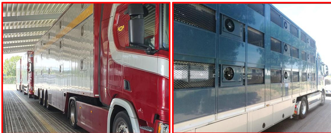
Forced-ventilated closed trucks (left) and trucks with perforated side walls (right) should be prohibited in the summer period as they impose a higher risk of heat-stress
