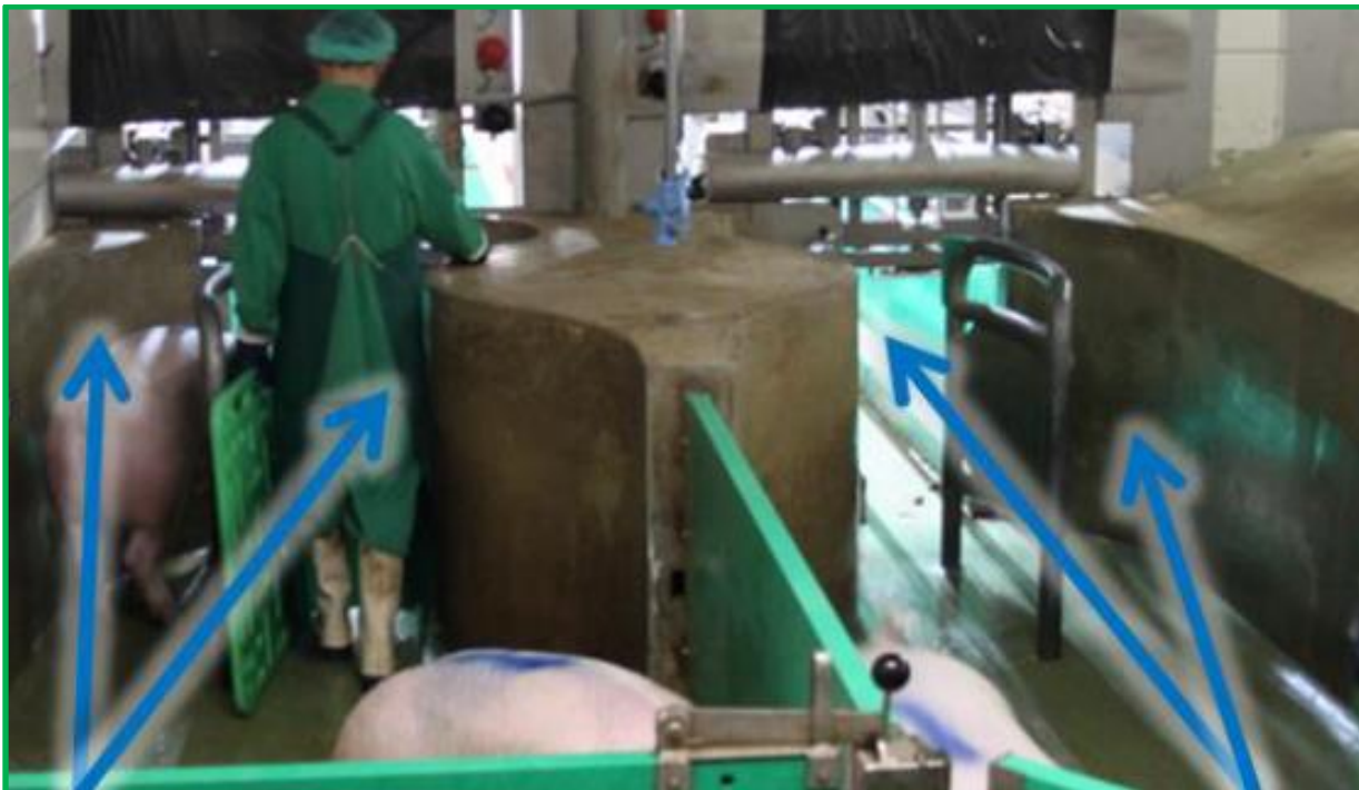
Double-entrance to the raceway to reduce stress at Grossfurtner (AT)
