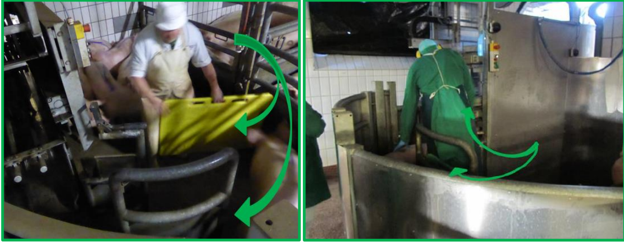
Double-entrance to raceway to reduce stress at Naturverbund (DE) and Grossfurtner (AT)
