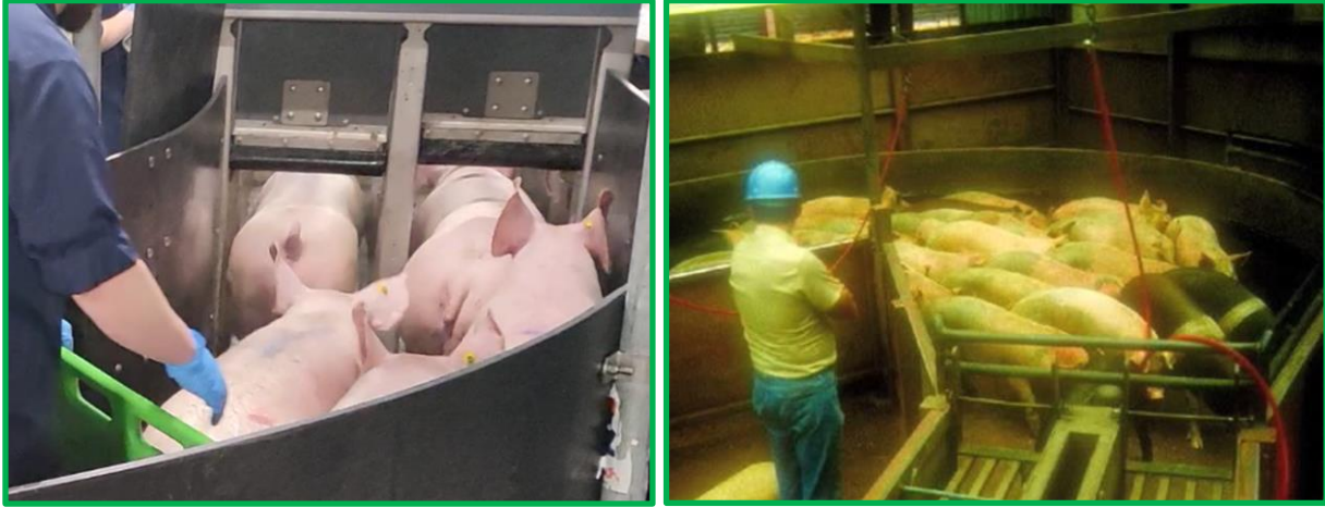
By installing two single-file raceways next to each other, pigs can choose between the left or right entrance and feel less pressured. Photo on the left: Compaxo in Zevenaar (NL). Photo on the right: © T. Grandin
