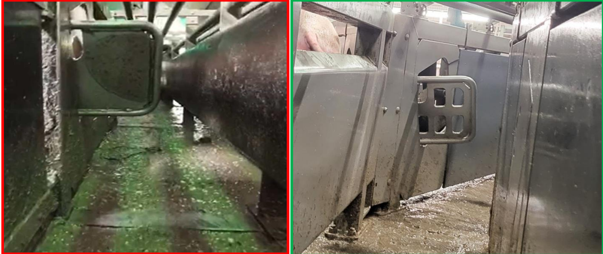
At Compaxo in Zevenaar (NL), the old anti-reverse doors (left photo) were replaced with see-through anti-reverse doors (right photo) that have small holes in them, allowing pigs to see other pigs ahead.
