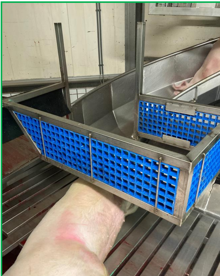
A “barrier trap” (in blue) to prevent pigs that were not stunned correctly by the automatic stunner from “escaping” and running around in panic. Emergency manual stunning can now
