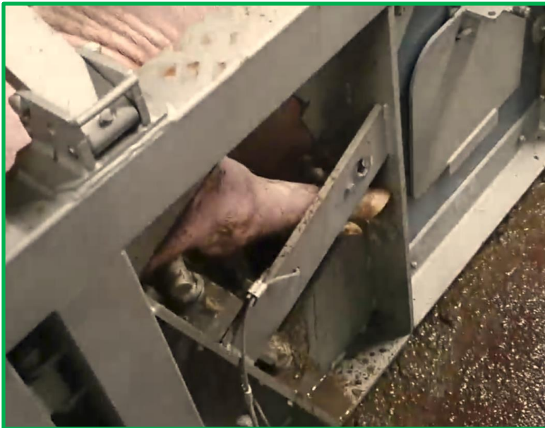
Pig with his/her leg caught in a gap next to the anti-reverse door
