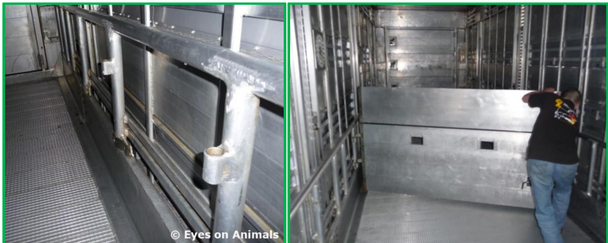
Trucks with partitions that can be placed in different positions, so that different size compartments can be created.
