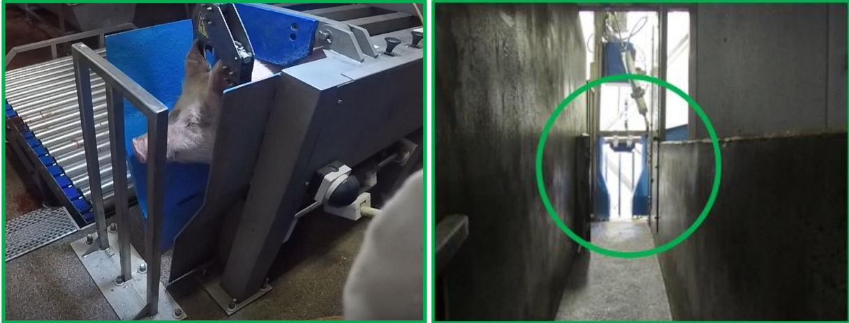
Restraint box in the new situation: box opened at the front. The pigs will have less fear to enter this raceway as the end appears open, as if they will be able to exit it up ahead.
