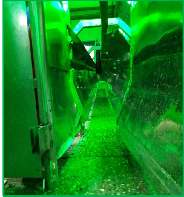
Left: old situation with open sides, right: new situation with solid sides and green light. Due to the solid sides workers cannot be seen anymore. Lighting however has increased reflections.
