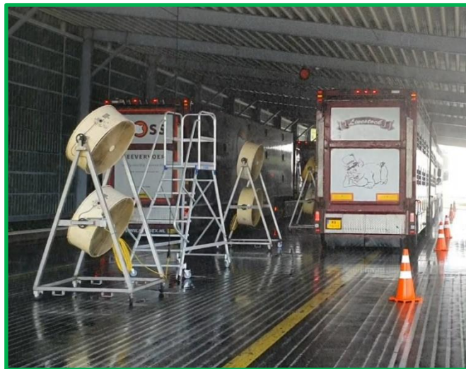
Left, old situation: fans are too low, the airflow does not reach the top decks. Right, new situation; two fans are stacked and can be set at different angles so also upper decks can be reached.
