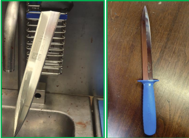
Use a knife blade of 16cm minimum with a cutting edge on both sides.
