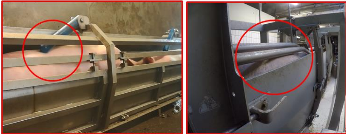
These raceways are too low: the pigs' backs are rubbing against the top of the raceway. There is a big chance these pigs feel trapped, refuse to move forward and will try to walk backwards to get out.
