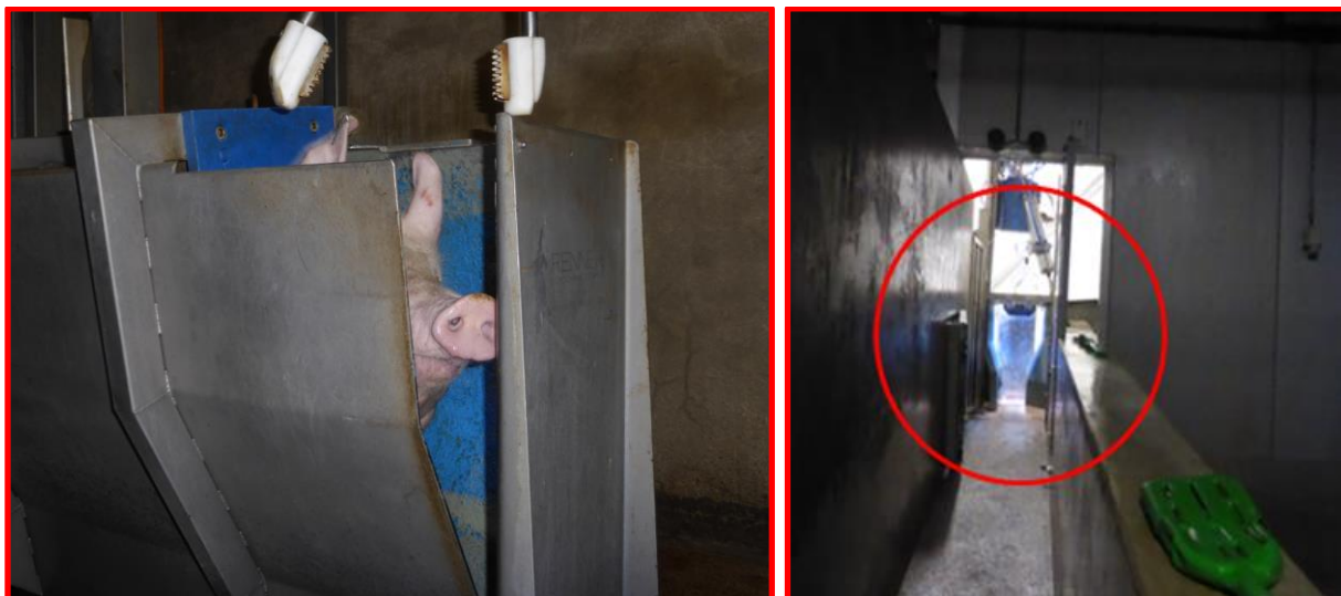
Restraint box in the old situation: closed front. Pigs will be scared to enter this raceway as it appears dead-ended.
