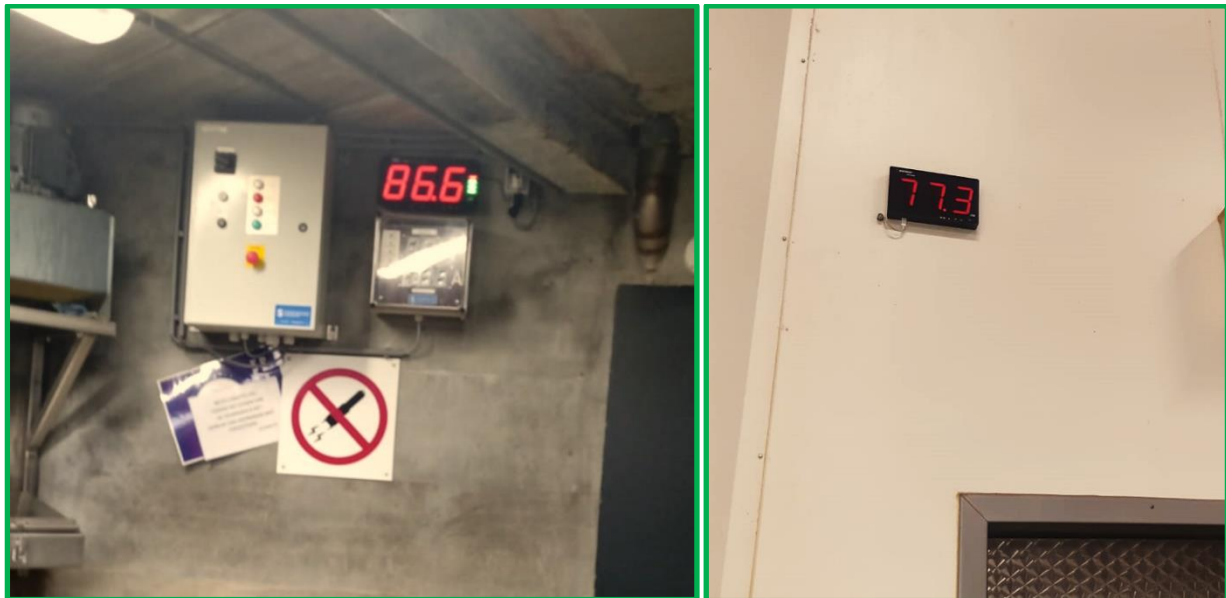
Decibel monitors in Dutch slaughterhouses. Left: 86.6 dB at the unloading dock, right: 77.3 dB in the lairage.
