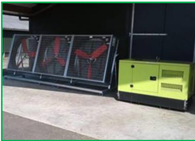
Large mobile fans to ventilate stationary trucks help reduce heatstress
