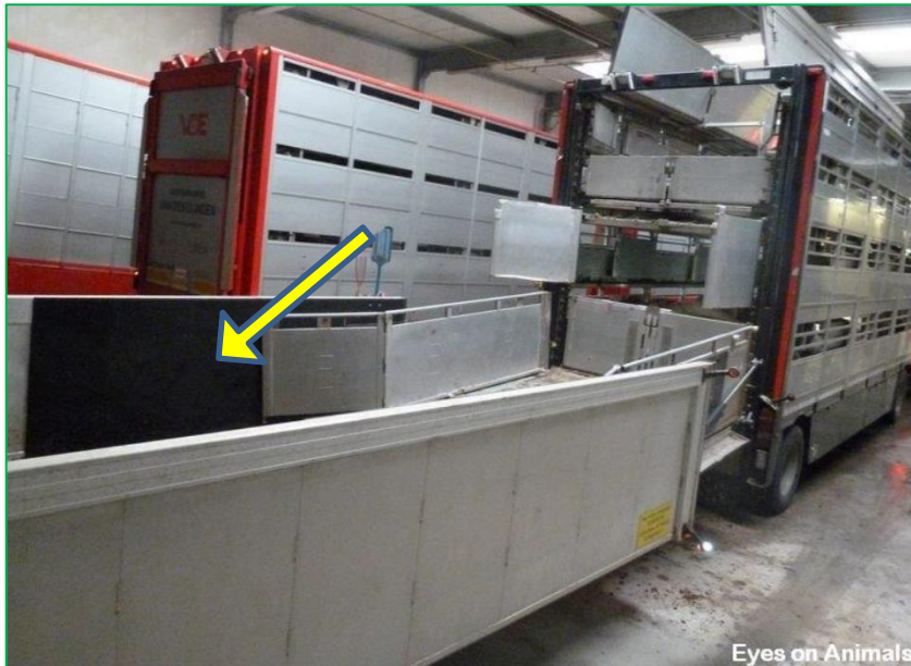
Rubber panels to reduce noise
