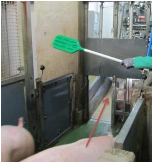
A raceway with a slope going upwards makes it difficult to move the pigs
