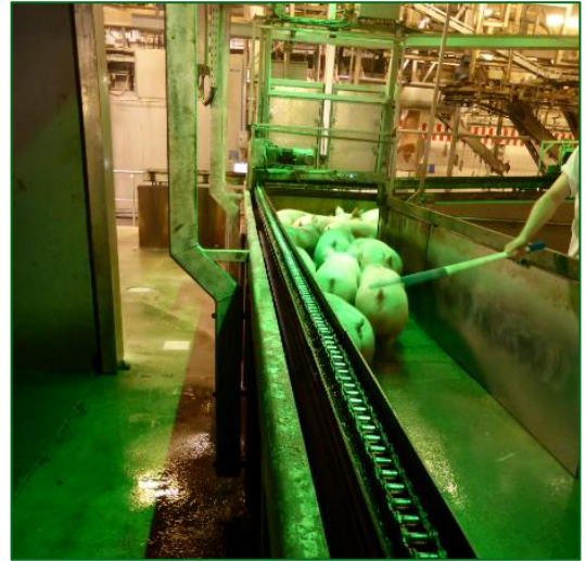
Green lighting was installed at Tönnies to reduce the creations of shadows.
