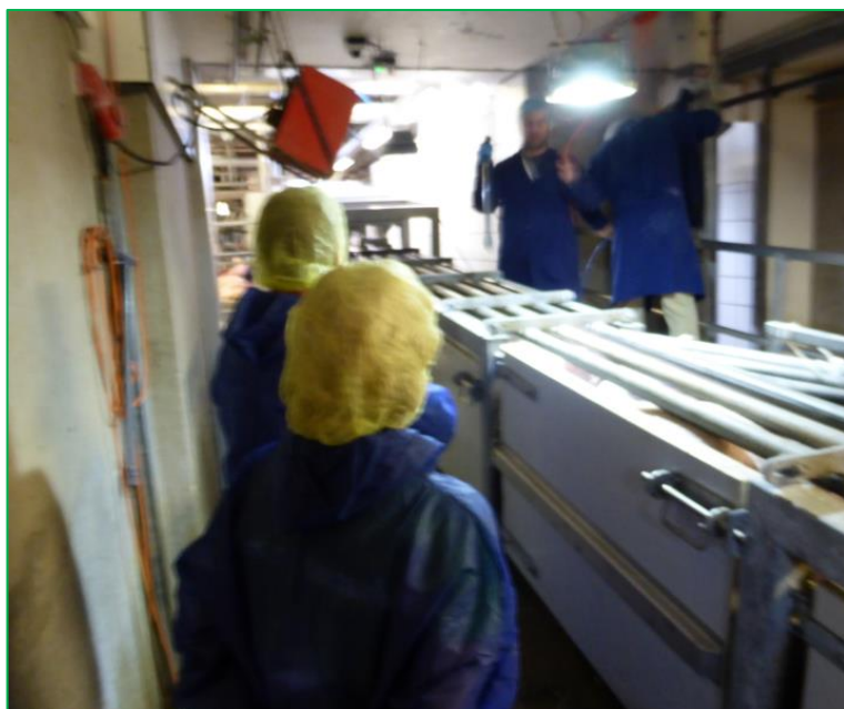
Compaxo placed extra lighting above the passageway. The result: the pigs are a little less stressed and walk forward more easily.
