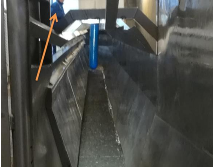
The worker at the end of the raceway can frighten and demotivate pigs to move forward. The blue anti-reverse door will also cause pigs to balk – it is a clear obstruction and colour contrast.
