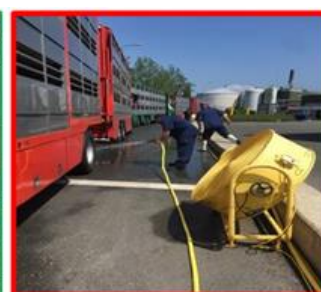
This ventilator is too short, the airflow doesn't reach the top level.
