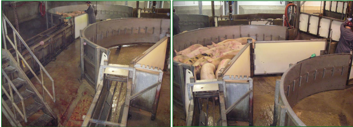
The Corral system. This design works very well according to Temple Grandin. There are however too many pigs in the Corral system on the photos. Temple Grandin recommends to only fill up half of the Corral system with pigs.
