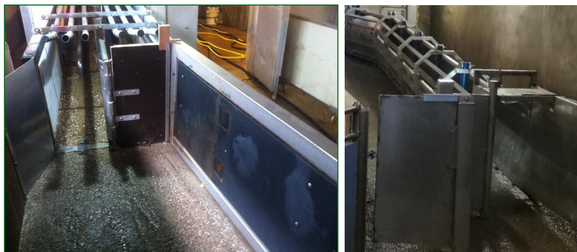
Raceways with a cage construction (see photos) work less well than raceways with an open top
