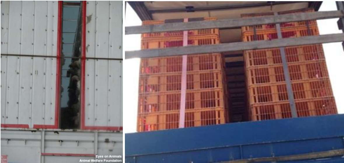
Truck with passage in the middle to improve air flow. Left: poultry Right: rabbits
