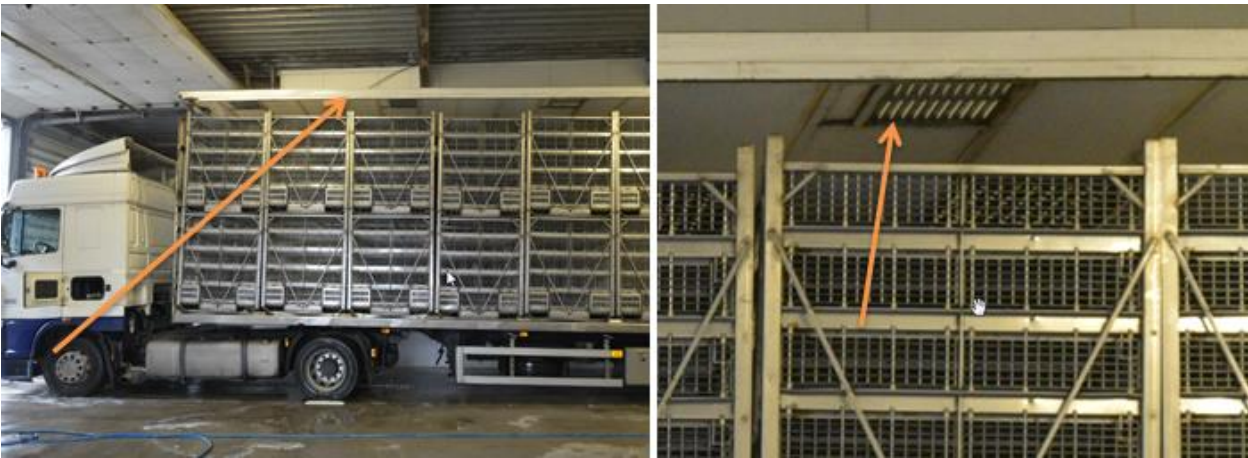
Truck with roof that can be raised and air vents in the roof to allow trapped warm air to exit.
