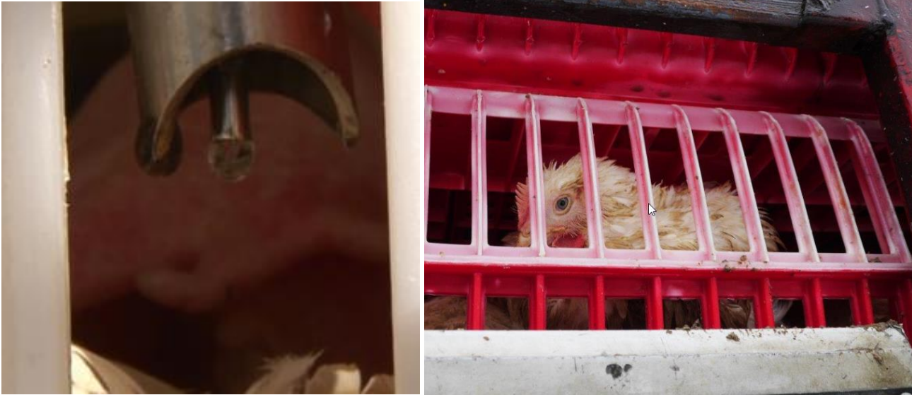
Leaking drink nipple in poultry transport
