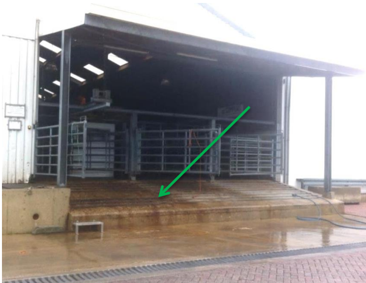
Figure 50. Loading dock with anti-slip ridges at Vion Food Group slaughterhouse.
